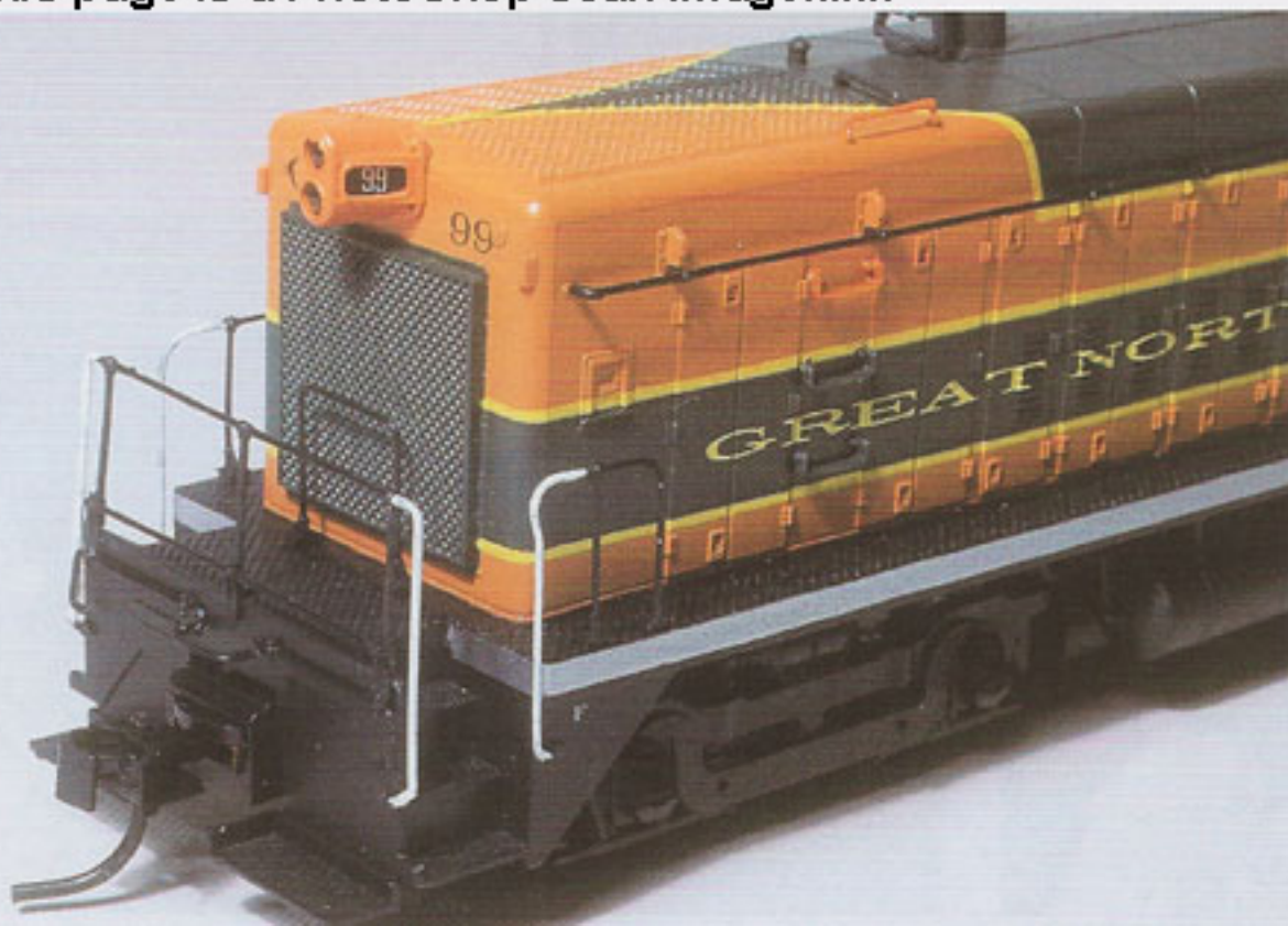
Fig. 8-23. Pactra's Racing Finish is a flexible paint that works well on locomotive handrails. Be sure to coat the entire handrail so the paint forms a jacket around the part.
