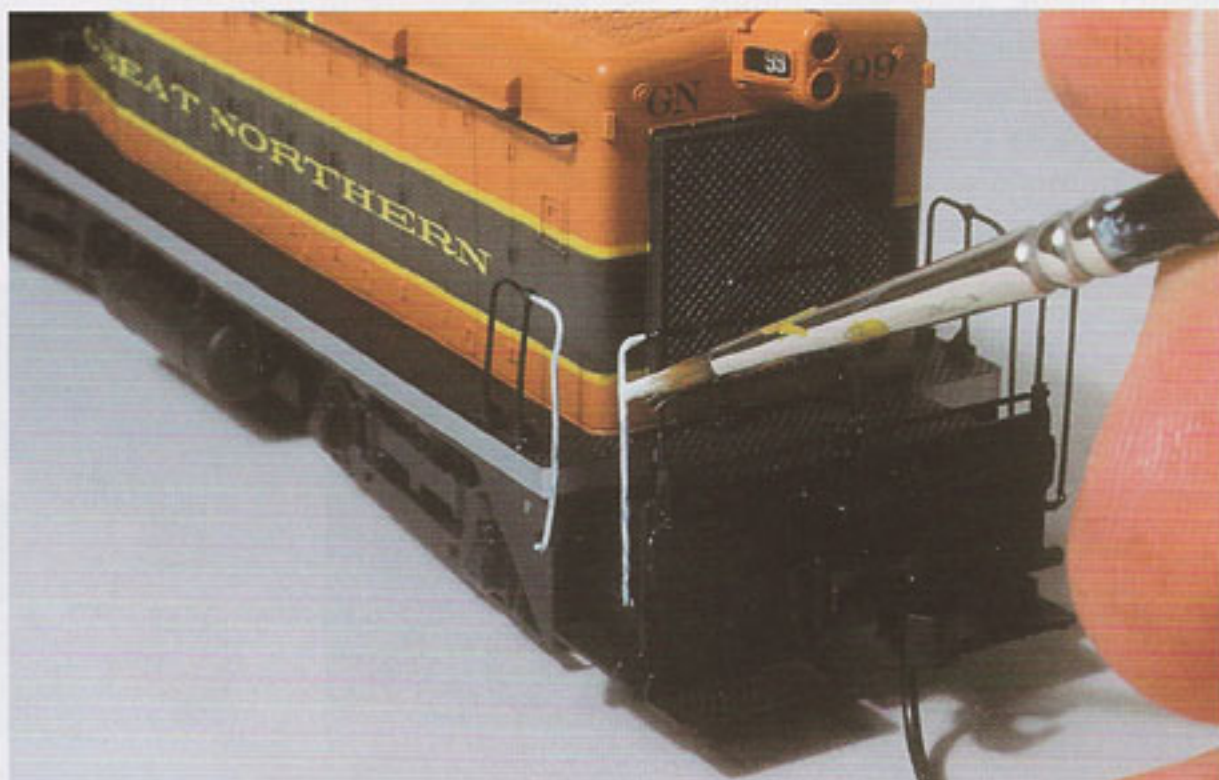
Fig. 8-23. Pactra's Racing Finish is a flexible paint that works well on locomotive handrails. Be sure to coat the entire handrail so the paint forms a jacket around the part.
